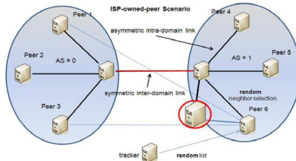
Fig. 4.1: Insertion of ISP-owned peer in pure BT.
